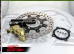
Cod. 305303 Rear brake caliper 4 pot kit
