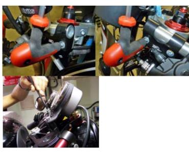
Fasten clip on bars with 22Nm. Fasten instruments.
