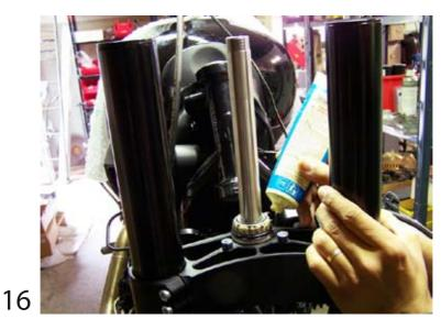
Insert bearing on new bottom trees. (Use waterproof grease on bearing)
