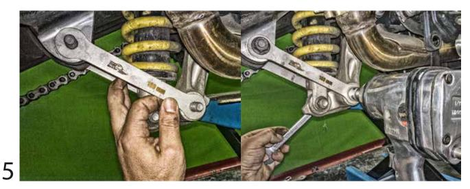
Insert right link rod and fasten.
