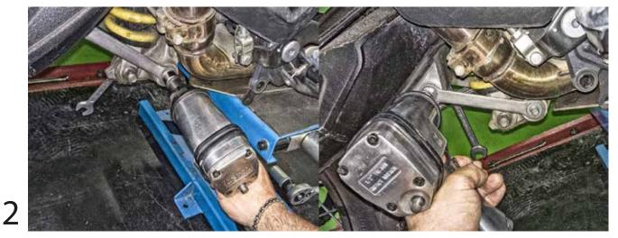
Remove nuts securing the connecting link rods of progressive system.
