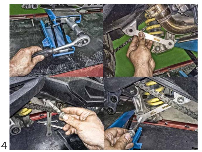
Lower motorcycle until the holes coincide. Install new link rod on left as photo.
