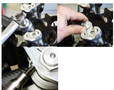
Fasten nuts with torque of 42 Nm. Fixing the upper plate 25 Nm.
