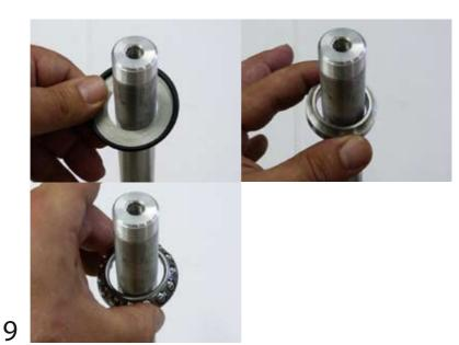
Insert first dust cover and bearings guide. Insert bearing (Lubricated on lithium grease).
