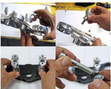
Remove the riser from the original plate, Attach the oem riser using the hardware supplied.
