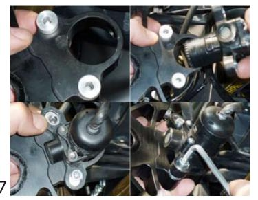
Install ignition switch on top plate (use spacers provided)
