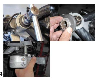
Unscrew the nut from axle and remove the bottom plate. Be careful during this step and get help to support the bike.
