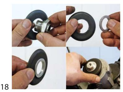
Insert bearing guide, pull off oem nuts from plastic dust cover and enter spacer provided.
