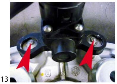
Remove the ignition switch from the original plate.
