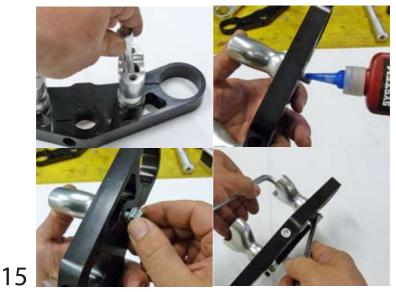
Attach the riser than keeping it parallel as possible. Add medium thread locker.
