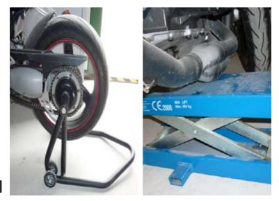
To support the bike using the rear stand, and to support the bike using the lower part of the headers, same a picture.
