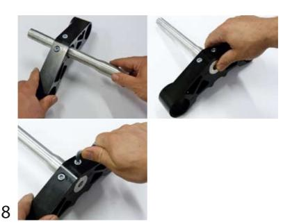
Insert and fasten axle to the bottom plate. Then tighten bolts to 25,5 Nm.
