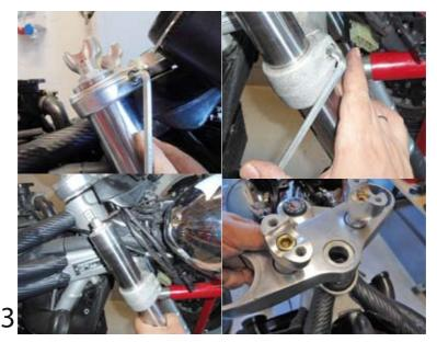
Slide off fork stems and remove top plate.
