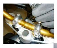
Reinstall the handlebar and set at 26 Nm Check riser bolts.
