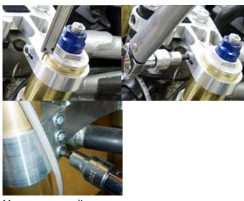
Measure stems slippage. Fixing the upper plate 25 Nm Bottom plate 15 Nm
