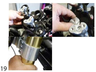
Mount the top plate and nuts on axle. Insert the fork stems.
