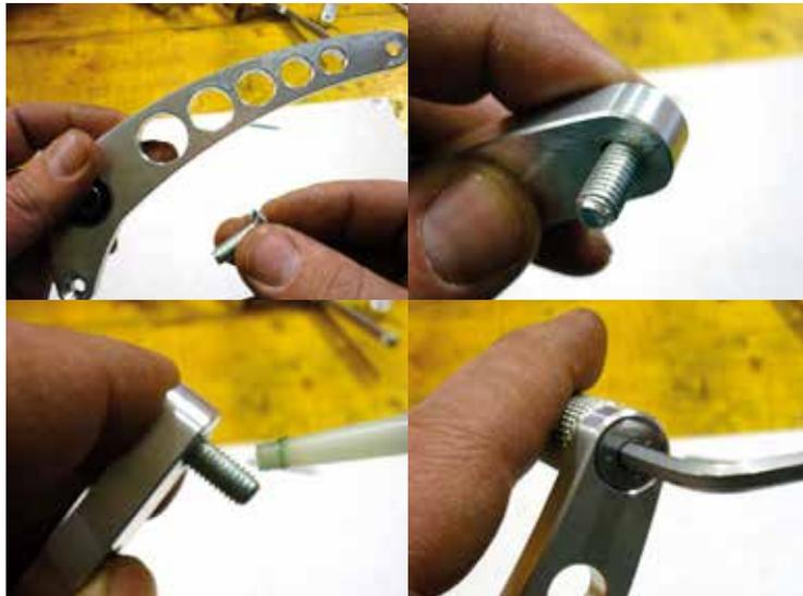
Insert the flathead bolt M6x20 add thread lock and tighten.
