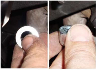
Insert first washer and nuts on bolt kit. Attention to the chassis VIN: 161318 and upcoming, changes the engine mounting bracket (Use M12 x 60 bolt, supplied in the kit)
