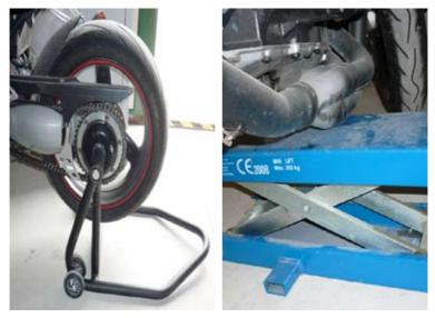
To support the bike using the rear stand, and to support the engine using the lower part of the headers, same a picture.
