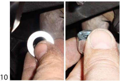
Insert first washer and nuts on bolt kit.
