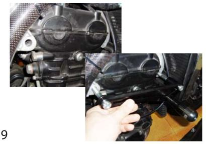
Insert 308512 right kit as in the pictures. Check for gaps between the frame and the engine unit at all right-hand mounting locations - if spacers were fitted originally they should eliminate any gaps, for avoid straining the frame when the mounting bolts are tightened.
