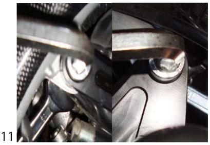
Fasten bolt and nuts, use tightening torques (50 Nm).
