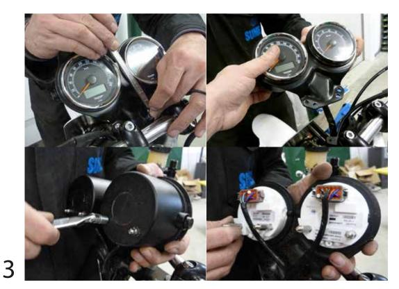
Remove OEM bracket and shell.
