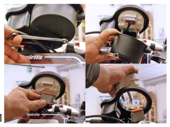
Remove the shell of the speedometer.
