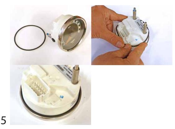
Apply O-ring on speedometer.
