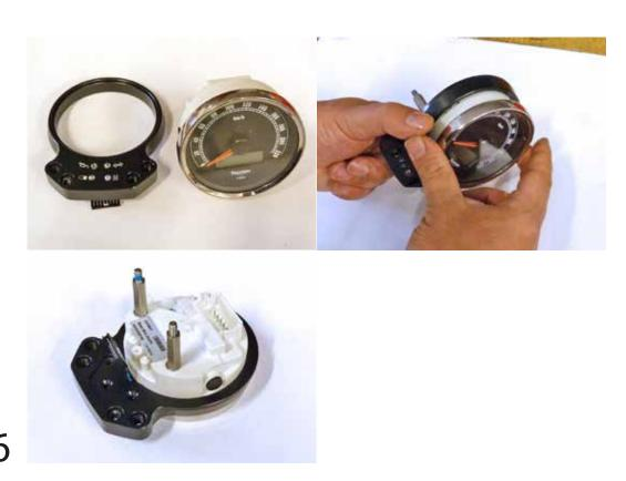
Insert the speedometer on the new bracket.
