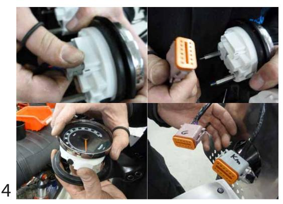
Pull the plug and remove instruments.
