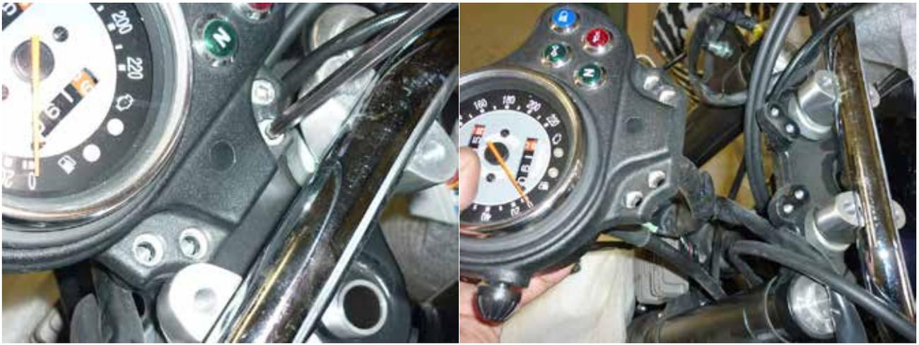
Remove instrument and handlebar.
