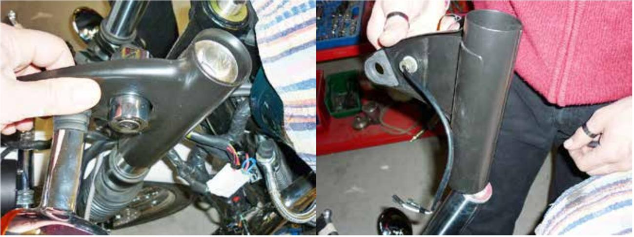
Slip off headlight brackets and remove ignition switch.
