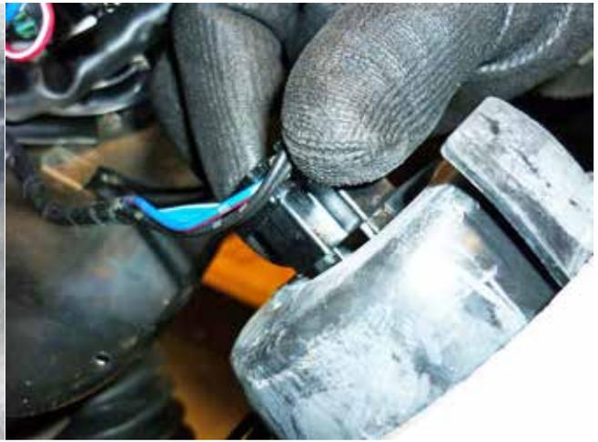
Remove ring and beam of the stock headlight and unplug the lamp.
