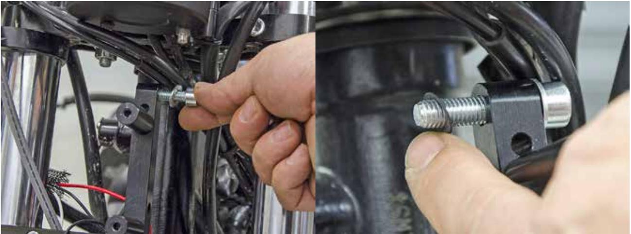
Insert allen bolt M8x35 with washer as photo.
