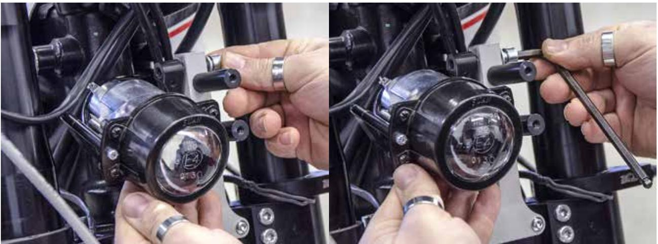
Fix headlight with the correct angle.
